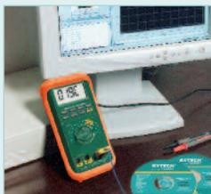
Optional Windows<sup>®</sup> 95/98/NT/2000/ME/XP compatible PC communication software and optically isolated cable for data collection.
