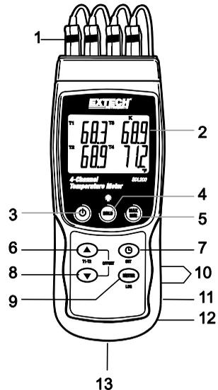
**Notes:** Items 10 – 12 are located behind the snap-off compartment cover on meter's right side.
