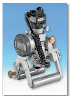
The ideal aid for depth measurement. The digital dial gauge measures the distance between two focal planes for no-contact measurement of hole depths in circuit boards or cell depths on anilox rollers and intaglio cylinders The measurement should be accomplished at very high magnification to limit the depth of field - a
