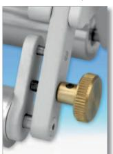
the only feature that allows exact recognition of the focal planes. The fine focusing mechanism can be pushed to the side for quick adjustment. An LED ring light is included with the set for materials such as rubber. The nine LED's are arranged at an angle of 30° to the optical centre.
