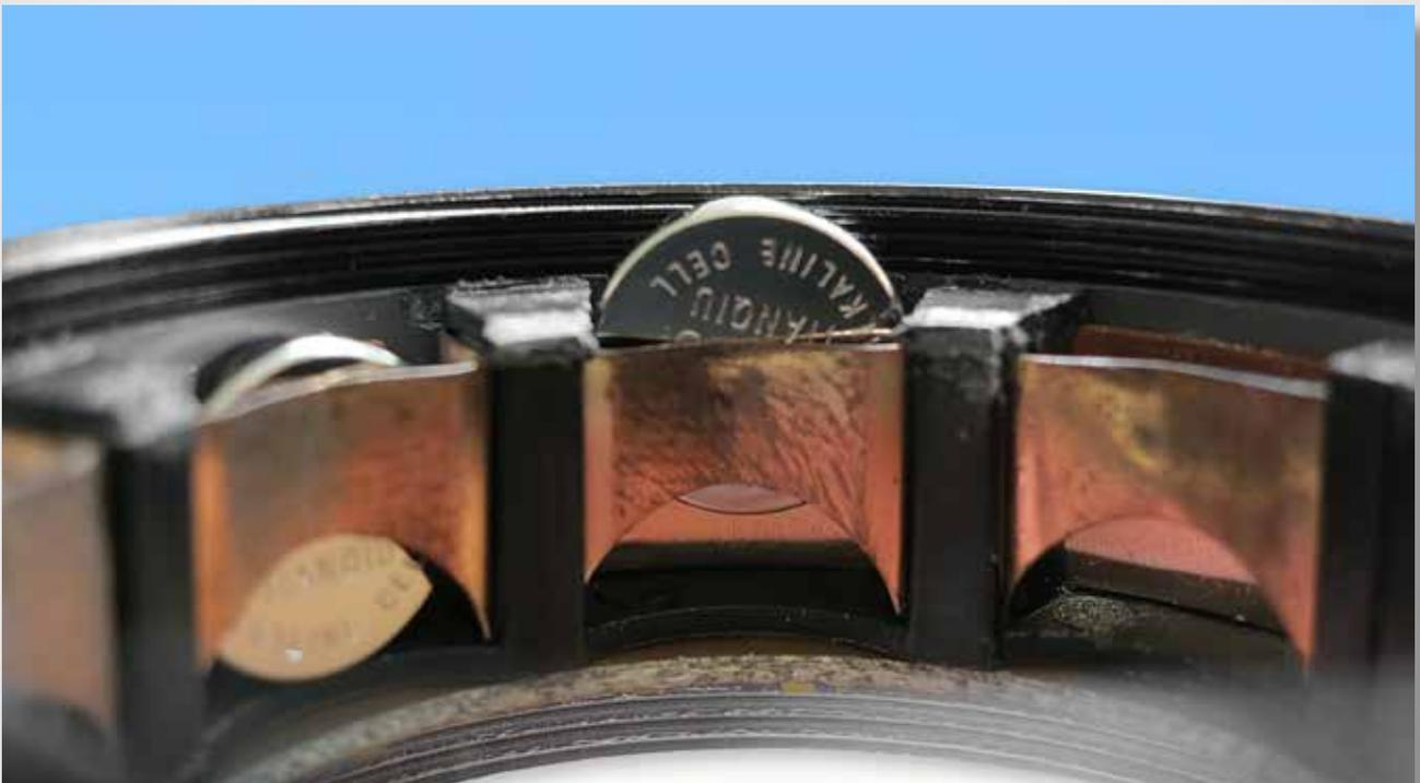
Now carefully slide the new batteries downwards into the retaining brackets. Reassemble all the parts and the battery change is finished.
