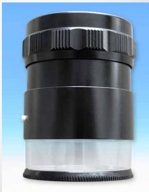
Carefully unscrew the upper part of the measuring magnifier.
