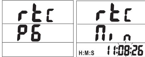
1. Press the SET button to access the setup mode
