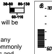
Normally, select the range in which the upper dB level is greater than any expected sound pressure level. The 60 to 110dB range is the most commonly used range. Use the 30 to 80dB range in quieter areas such as offices and classrooms.
