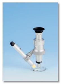
One of the primary advantages of the Peak 2034 series standard measuring microscope is its easy handling. Simply set the microscope on the field to be measured and focus – that's all. Thanks to the clear acrylic base the surface to be inspected can be viewed from all sides, making it easy to find the point to be measured. Focusing is accomplished by coaxial rotation of the tube. The short light path through the microscope makes the object appear reversed.
